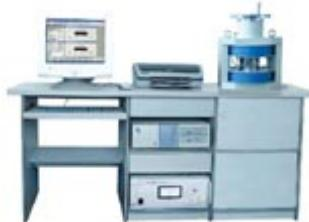
Automatic measurement on hysteresis loop and demagnetization curve of permanent-magnet material, accurate measurement on magnetic characteristic parameters such as remanence Br, coercive force HcB, intrinsic coercive force HcJ and maximum magnetic energy product (BH)max.
